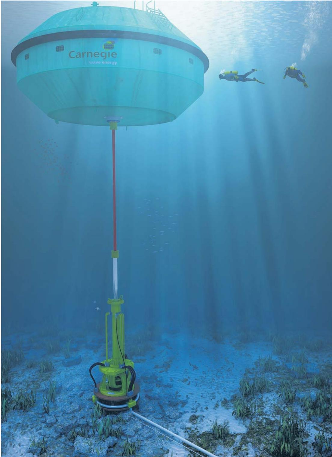
**Wave power: Waves heave buoys up to 4m, which then drive the pumps.**
