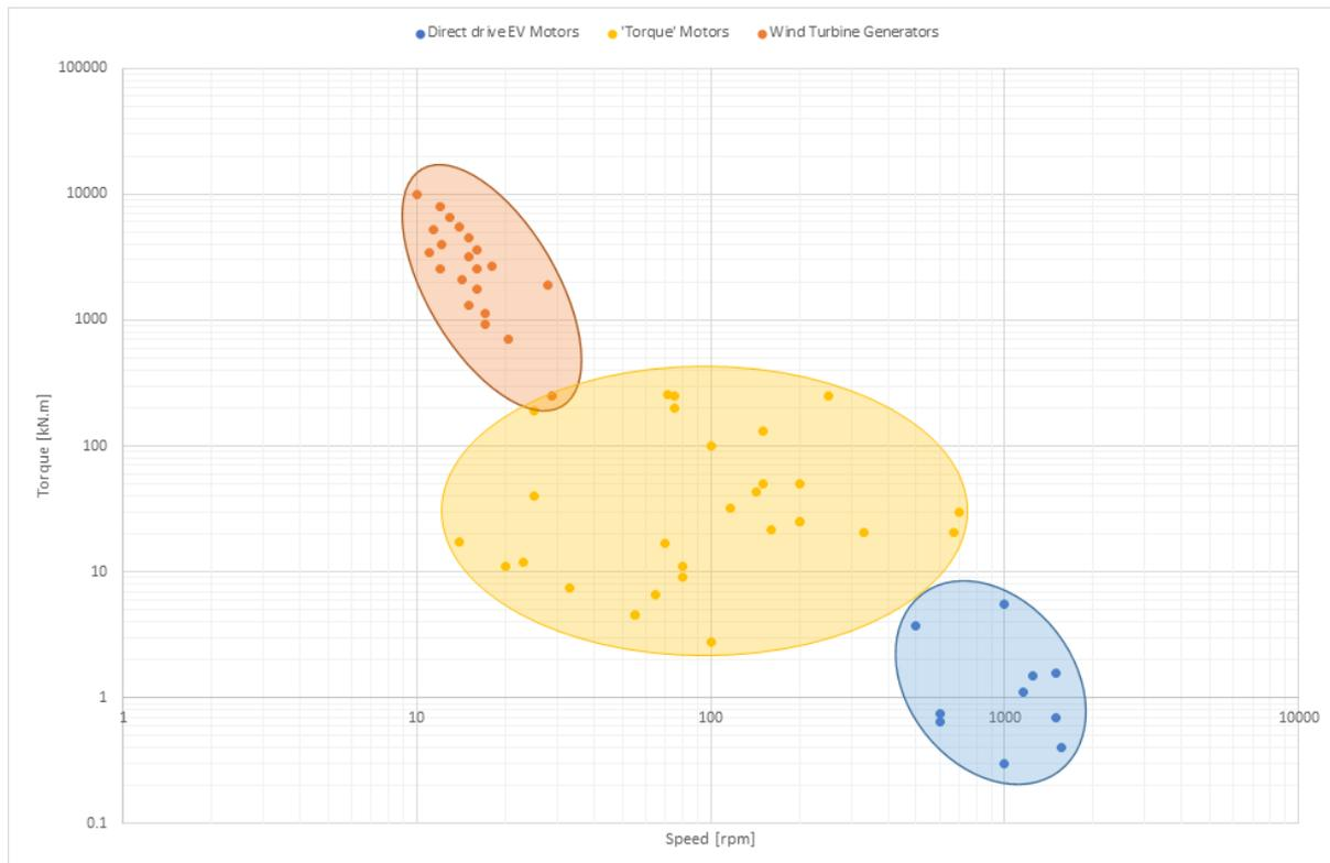
*Nominal torque vs nominal speed for 59 different electrical machines investigated for use in the CETO device across a wide range of scales*
