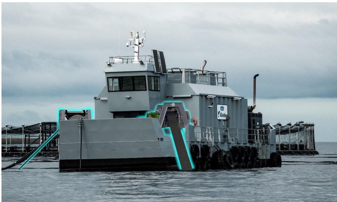
Artist's impression of Carnegie's new wave powered product incorporated onto a feeding barge utilised by the aquaculture industry
