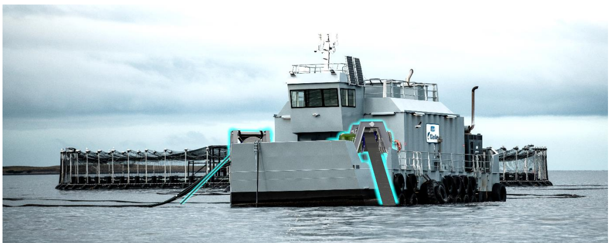
Artist’s impression of Carnegie’s new wave powered system incorporated onto a feeding barge utilised by the aquaculture industry (system highlighted on barge)
