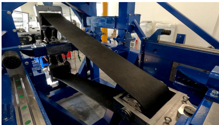
Belt testing at the IMPACT test rig at VGA s.r.l Italy
