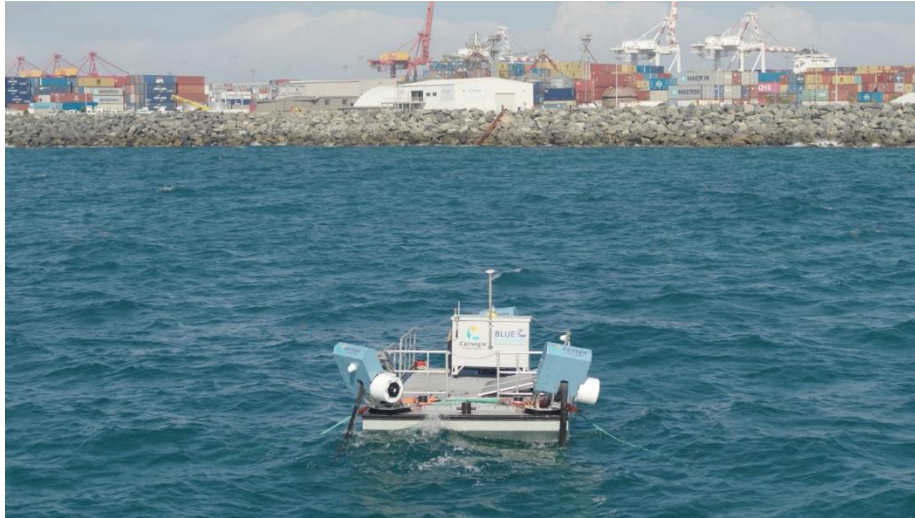
MoorPower in operation at the offshore test site in North Fremantle, WA
