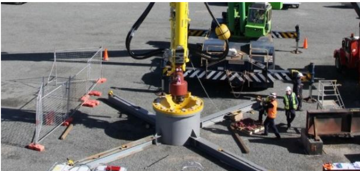
The SRP designed CETO 5 connector (red component in centre) during onshore testing, 2015
